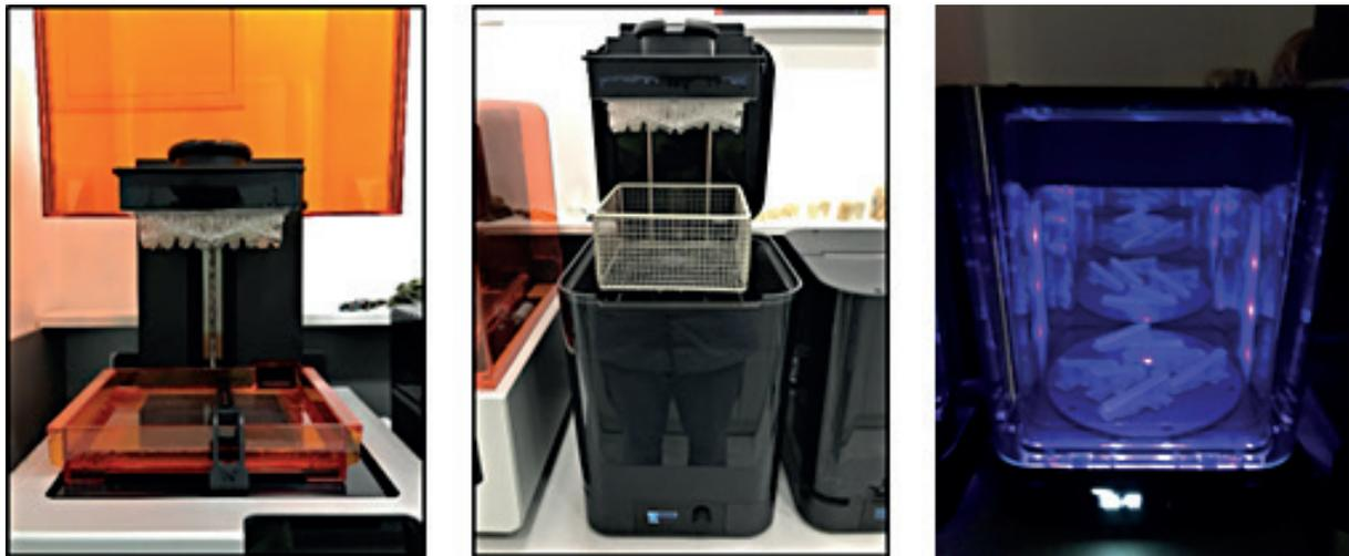
Figure 4. (a) Form 2 3D printer; (b) Form Cure Ultrasonic Bath; (c) Form Cure ultraviolet curing device
