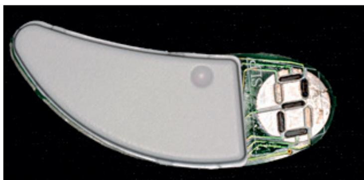
**Figure 2.** BiteStrip® portable electromyograph
