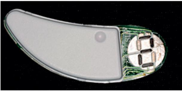
**Figure 1.** BiteStrip® portable electromyograph
